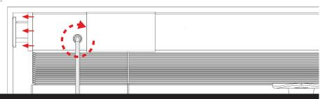
4. Slide the shrouds on the right and left of the headrail to cover the Allen wrench hole and the end cap grip.
