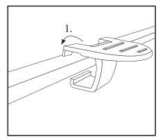
Once the teeth catch the lip on the top side of the rail while making sure the clip is resting against the rail, firmly push on the arm.
