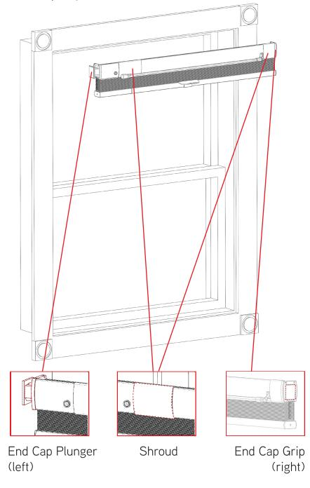
1. Push the plunger in firmly so the End Cap Grip (right) of the blinds fits into the window frame.
