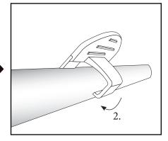
The arm will begin to flex and will slip below the bottom of the rail. The arm will catch the lip in a channel on the bottom of the rail. The clip will snap into place and will be ready to help raise or lower the shade.
