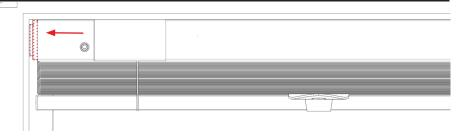
2. Allow the plunger to extend so the blind is flush with the top edge of the window.
